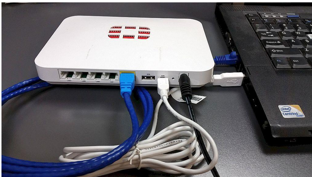
Figure 4.2: Firewall device connection to computer for configuration
