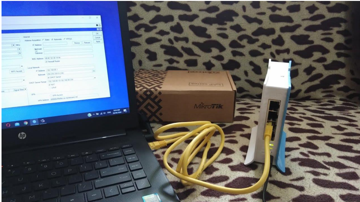
Figure 4.7: Mikrotik hAP lite TC device connected by laptop, accessing via WinBox
