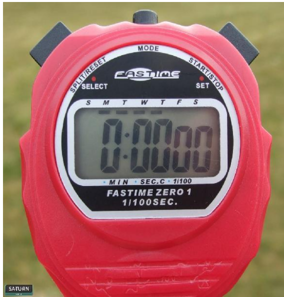
Stopwatch: Measuring observed time at the time of time study.
