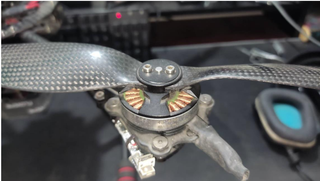
Fig. 3-5. Mounting motor and propeller on UAV arm
