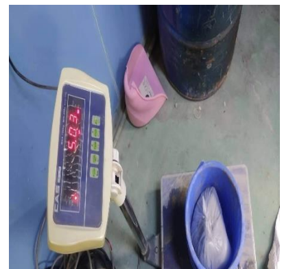
Figure 17: Measuring Stone sand Cement and water for concrete mixture
