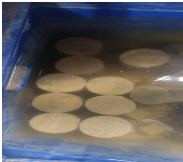
©Daffodil Internatio... Figure 23: Molds curing tank for curing
