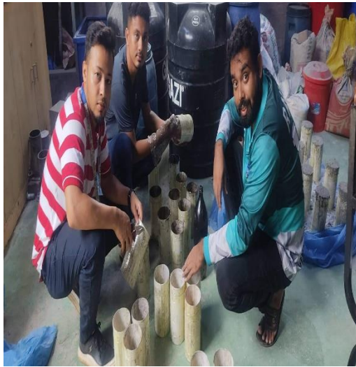
Figure 15: Mobil coating inside the cylinders
