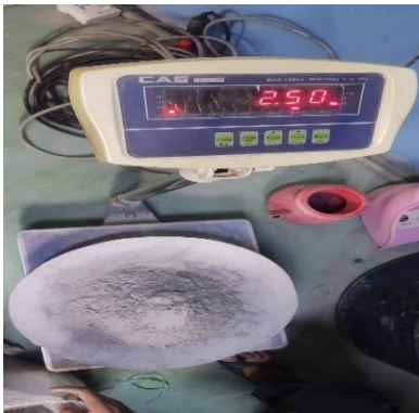
Figure 17: Measuring Stone sand Cement and water for concrete mixture
