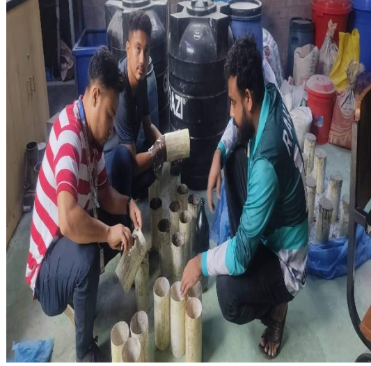
Figure 15: Mobil coating inside the cylinders
