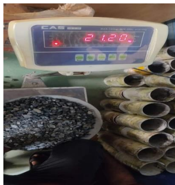
Figure 17: Measuring Stone sand Cement and water for concrete mixture
