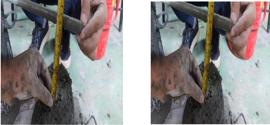
Figure 21: Taking Slump test result
