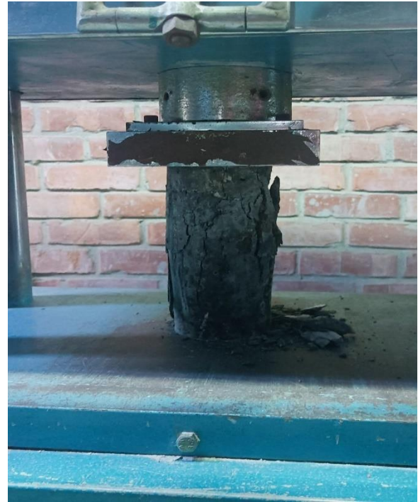
Figure 3.14: Compressive Test process is going on UTM and Failure surface under Compressive load
