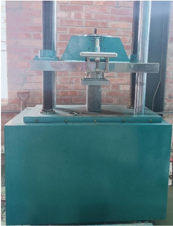
Figure 3.14: Compressive Test process is going on UTM and Failure surface under Compressive load
