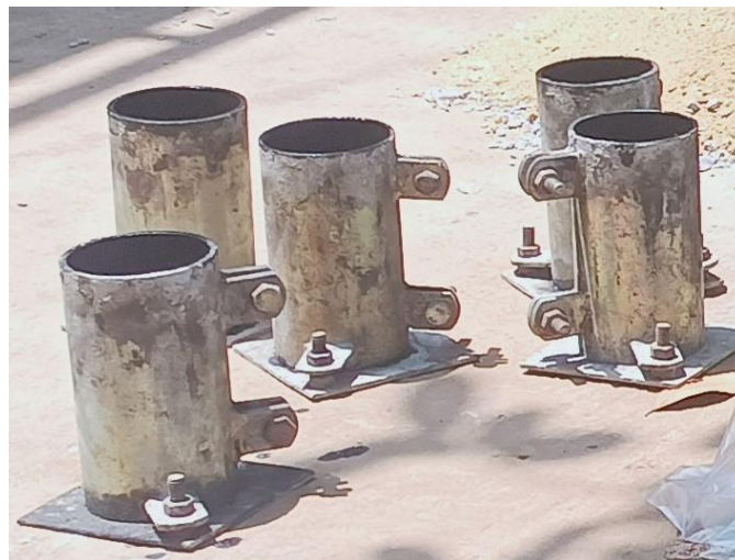
Figure 3.2: 4 inch × 8 inches of size of cylinder
