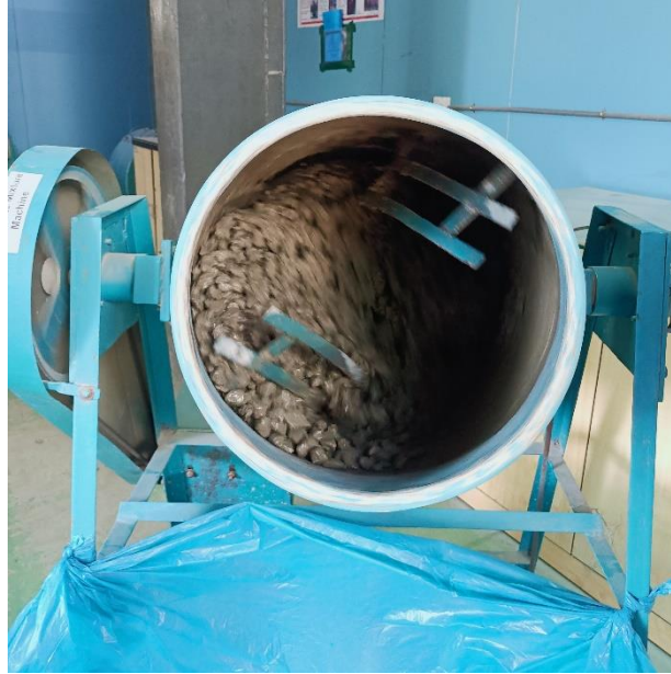
Figure 2.1: Machine mixing of concrete
