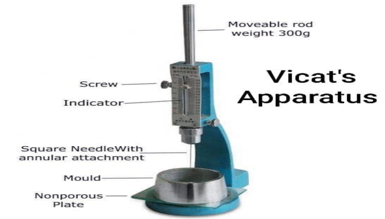
Figure 3.7: Vicat's Apparatus for Initial Setting Time Test
