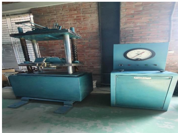
Figure 3.8: UTM machine for compression strength test
