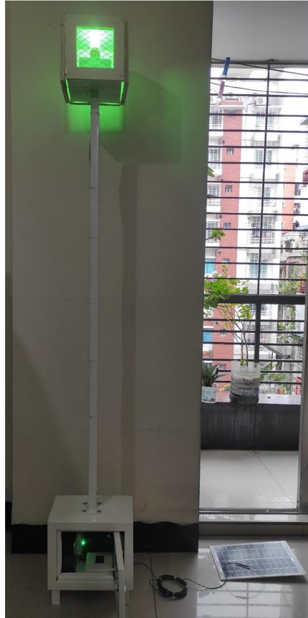
Fig. 7 Complete setup for mosquito trap with solar panel, Green SMD-LED and shock trap.
