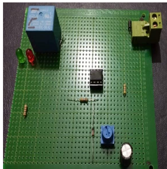
Fig. 5 Battery charge controller circuit.
