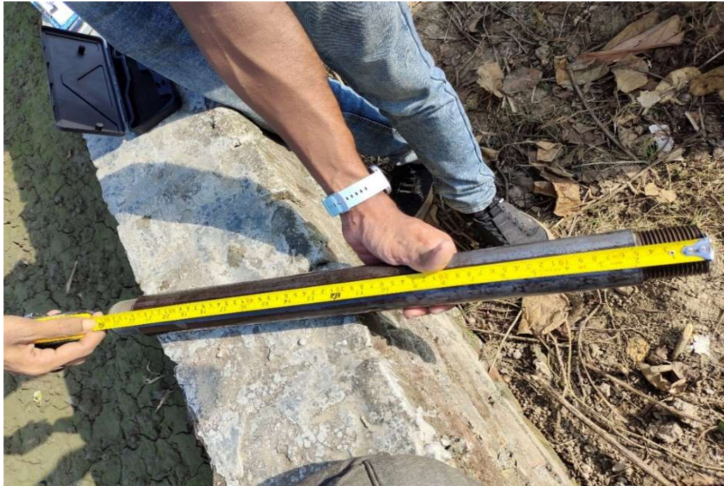
Figure 3. 6: Length Measurement of Split Spoon Sampler
