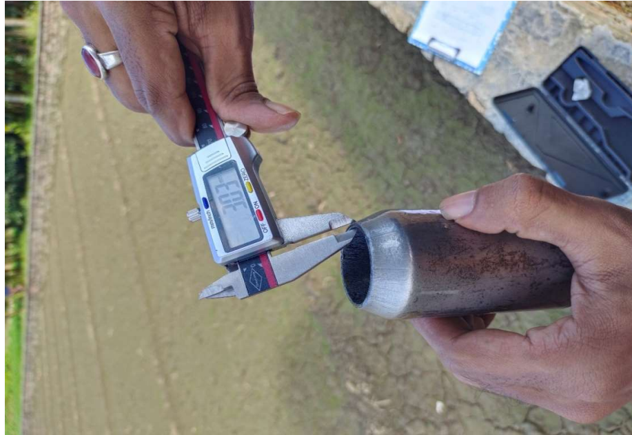
Figure 3. 7: Thickness Measurement of Driving Shoe
