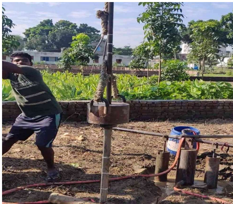
Figure 2. 7: Marking The Anvil and free free-falling height Measurement Auto & Manual Hammer
