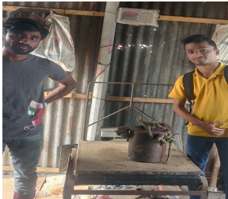
Figure 3. 3: The hammer is accurately measured in kg by digital weight machine.
