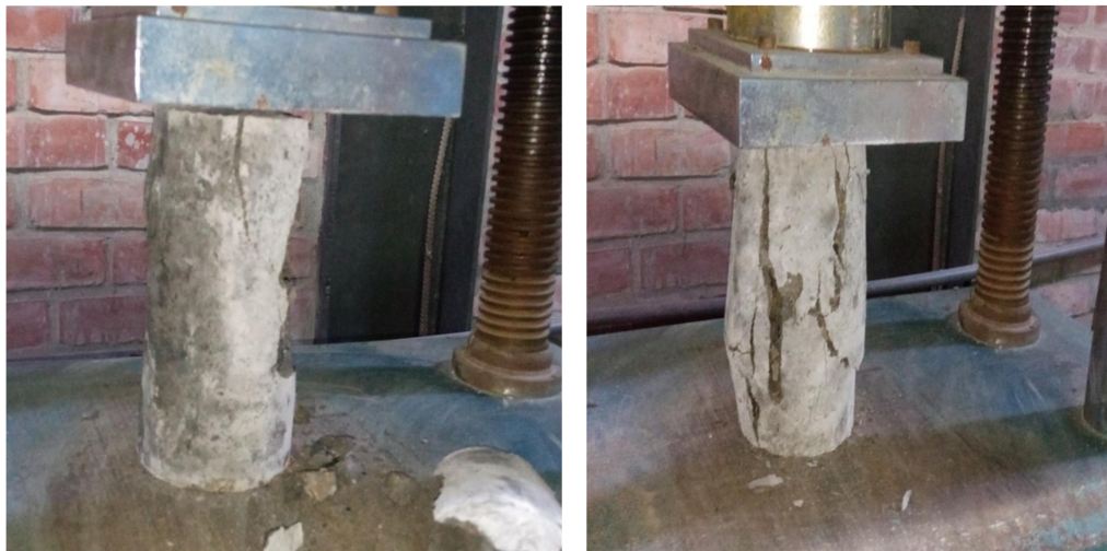
Fig 3.8: Concrete cylindrical compression Test
