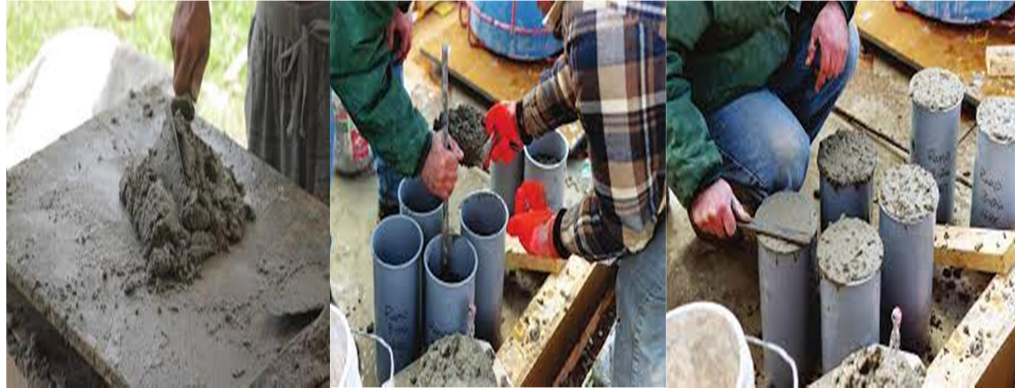
Fig 3.6: Concrete casting in the cylindrical
