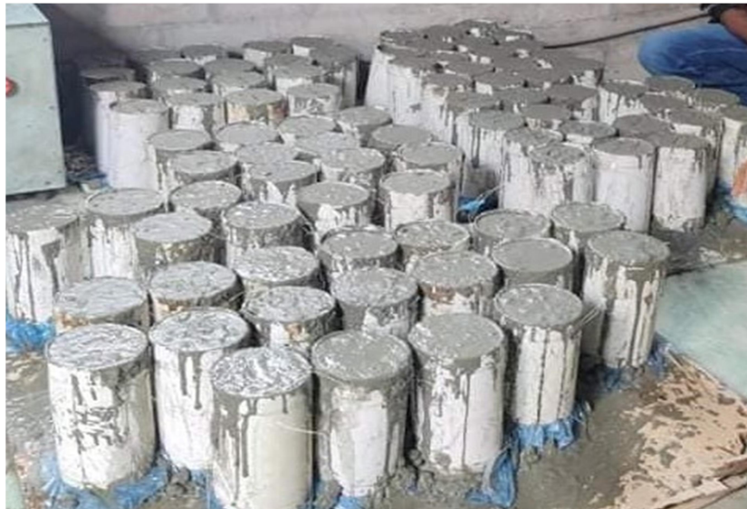
Fig 3.7: Concrete casting finishing works in the cylindrical
