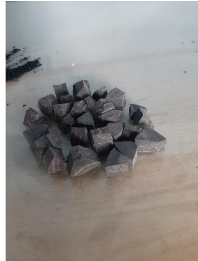
Fig.3.5 Coarse Crumb Rubber
