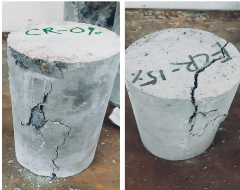
Fig.4.2 Cylinder after compressive strength test
