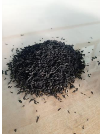
Fig.3.2 Recycled Crumb Rubber
