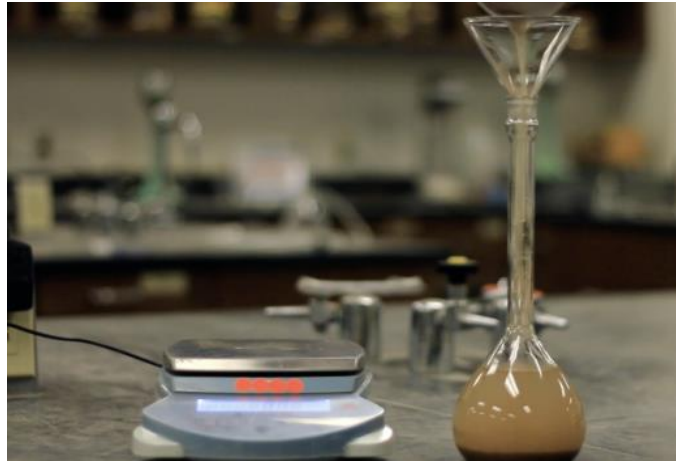
Fig.3.6 Determination of specific gravity
