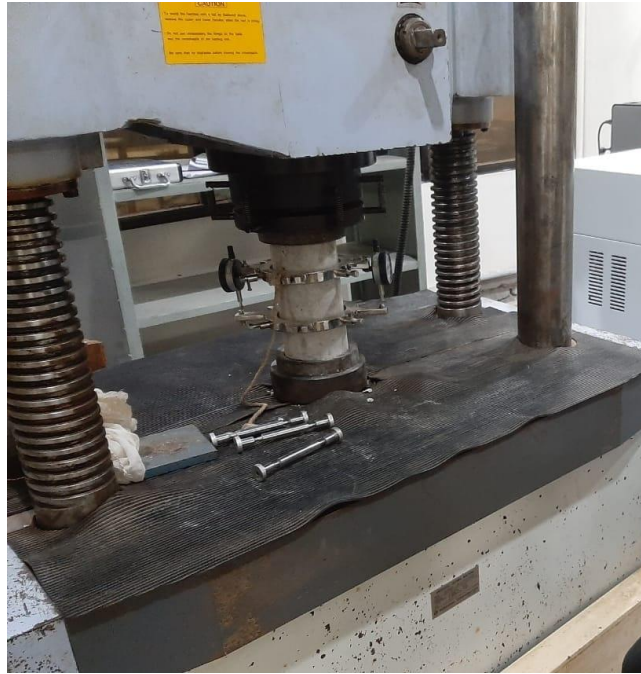
Fig. 3.9 Compressive strength test set up
