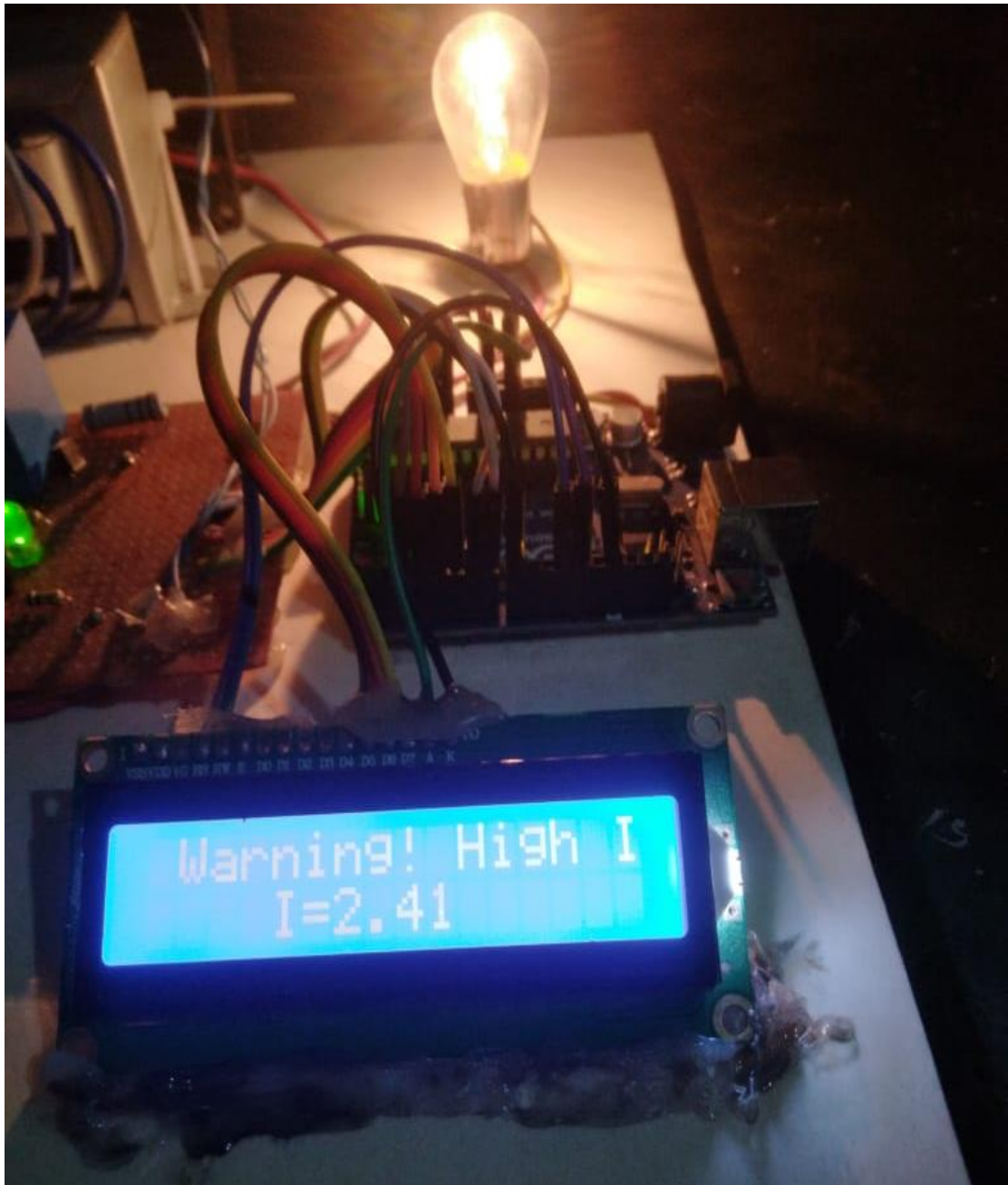
Figure 4.3: Giving warning for high current
