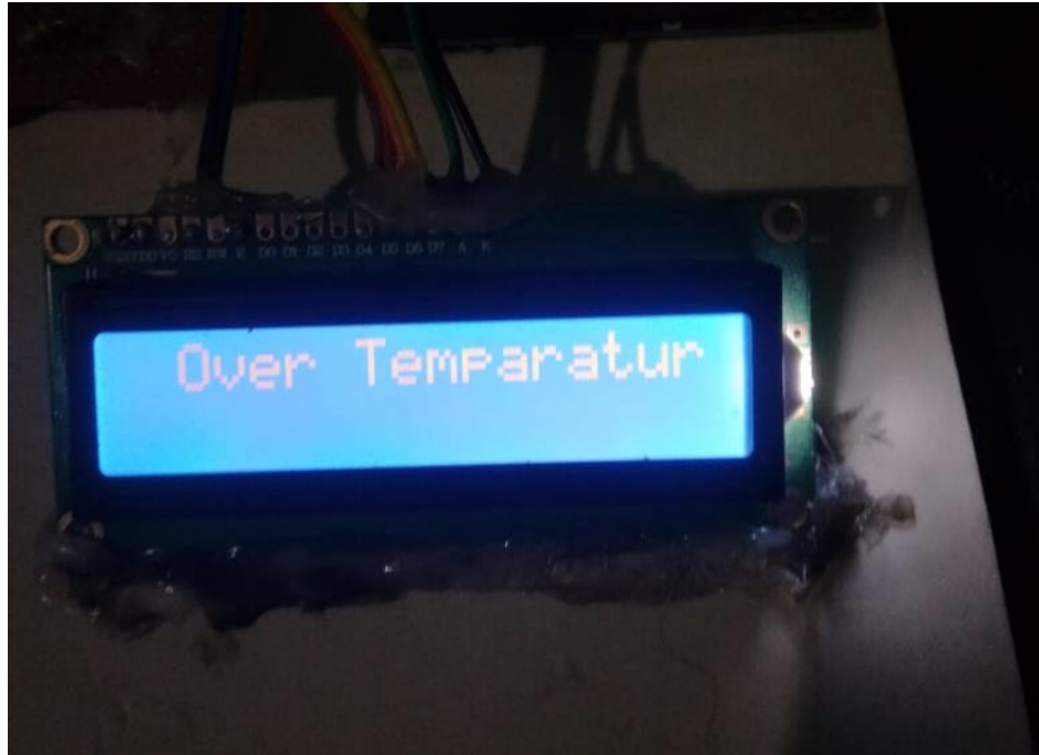
Figure 4.6: Over temperate ( T > 60 ) load gets cutoff and colling fan is turned on
