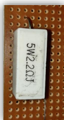
Figure2.3: A very low resistance to measure current (CT)
