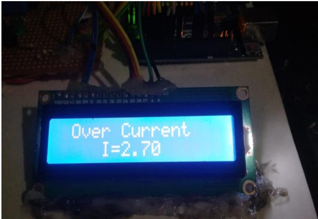
Figure 4.4: Over current and load get's cutoff
