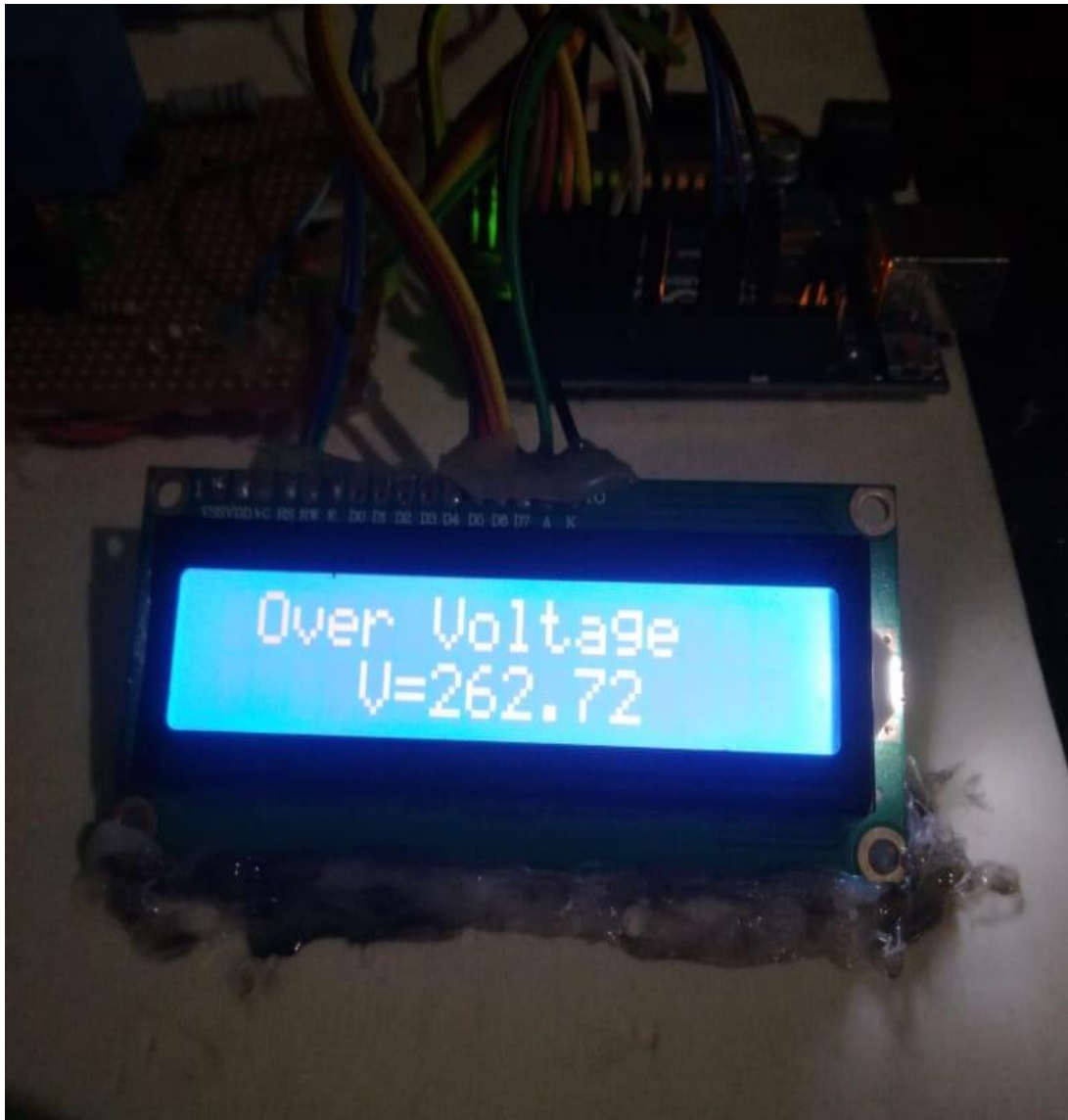
Figure 4.5: Over voltage ( V > 250 ) so load gets cutoff
