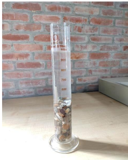
Figure -4.1.2: specific gravity Test
