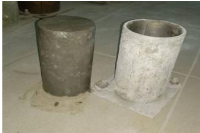
Figure 3.10: Opening cylinder Specimen from Molds
