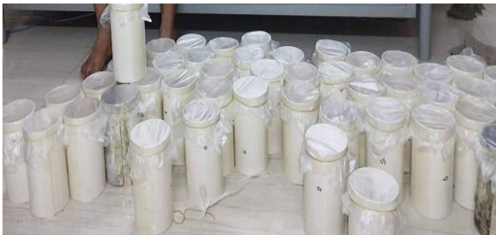
Figure 3.8: Molds for concrete casting
