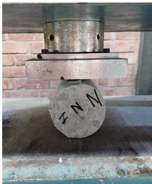
Figure 3.17: Compressive Strength test of cylinder mold
