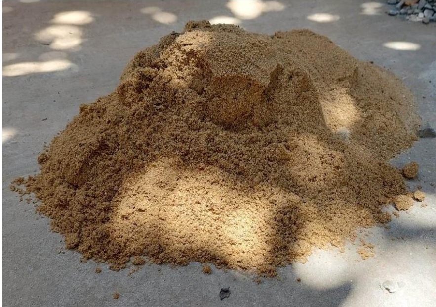
Figure 3.2: Fine Aggregate (Sylhet Sand)
