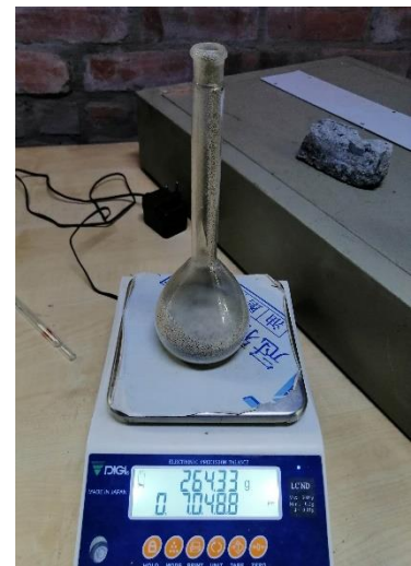
Figure -4.1.2: specific gravity Test
