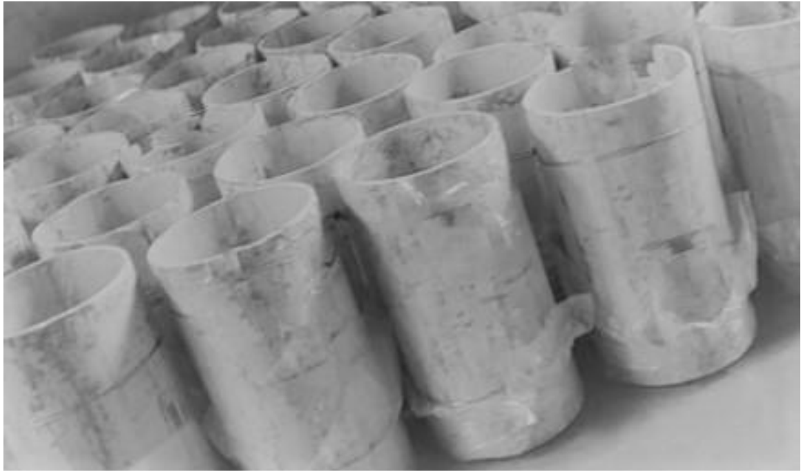
Figure 0-9: Plastic moulds prepared for casting concrete cylinder.
