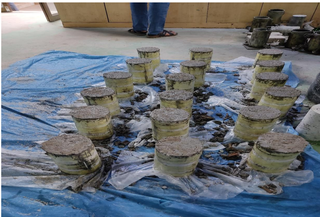
Figure 0-12: Casted mould for 24 hr
