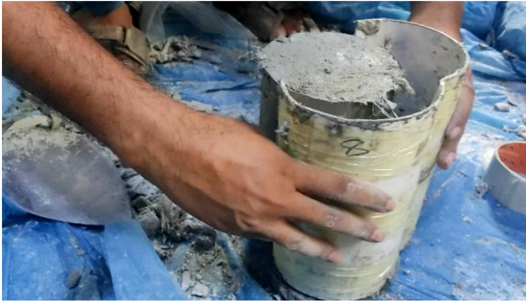
Figure 0-13: Remove the mould after 24 hrs
