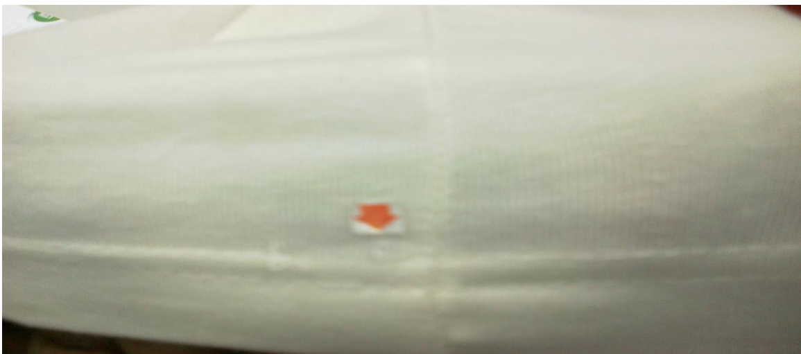
Figure: Unbalanced Stitch
