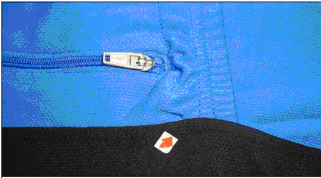
Figure: Seam puckering
