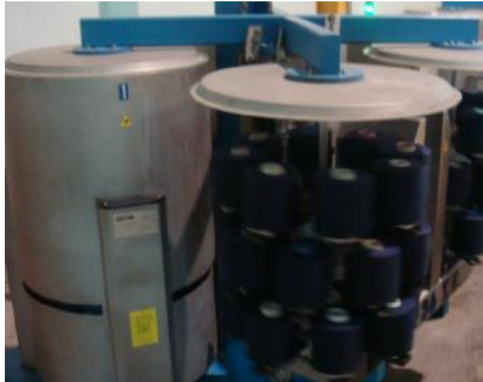
Figure-31: Package arrangement in dyeing machine
