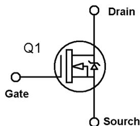
Fig 3.8 - N Channel MOSFET driver.
