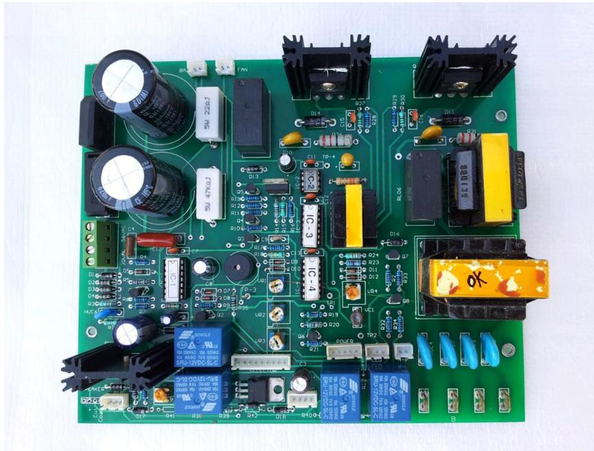
Fig 3.21 - Component Loaded Electro Surgical Diathermy PCB
