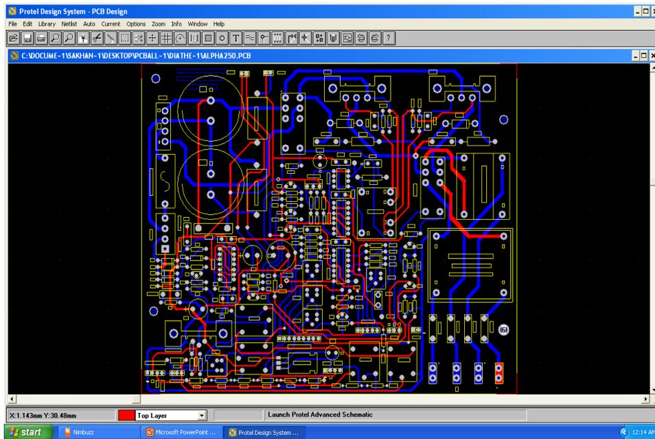
Fig 3.16 - Main PCB of Electro Surgical Diathermy
