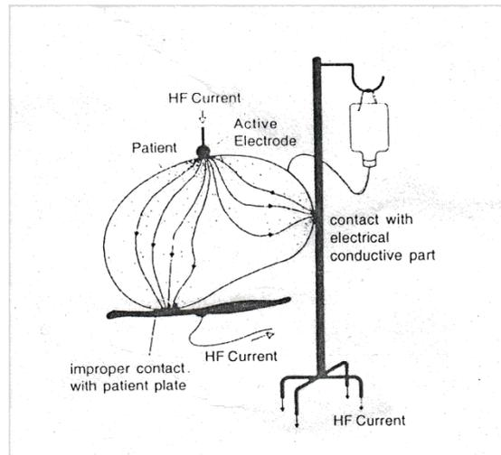
Fig 2.18- Contact with electrical conductive part.
