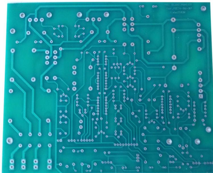
Fig 3.19- Bottom Side of Electro Surgical Diathermy PCB
