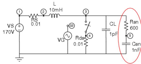
Fig 3.11 - Inductive Load Circuit with Snubber
