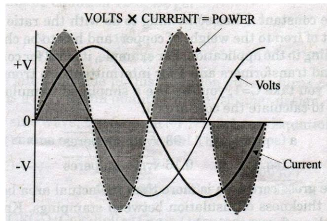
Fig 3.14 - The net power consumed in an inductance is zero
