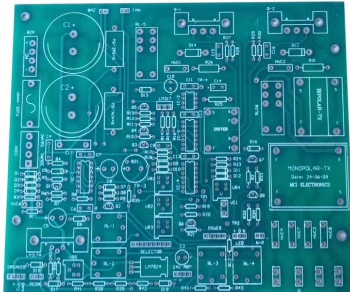
Fig 3.18 - Top Side of Electro Surgical Diathermy PCB
