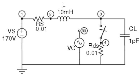
Fig 3.10 - Inductive Load Circuit
