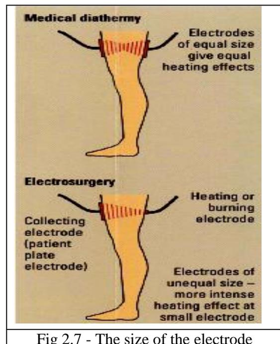
Fig 2.7 - The size of the electrode
