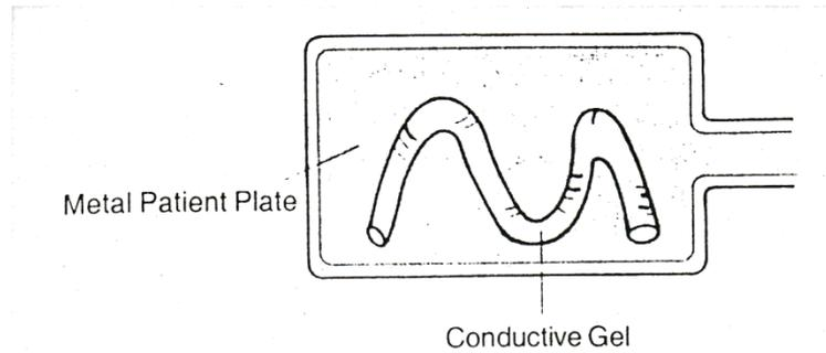
Fig 2.20 -Metal plate and conductive gel.
