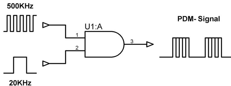
Fig 3.5 - Pulse duration modulation circuit
