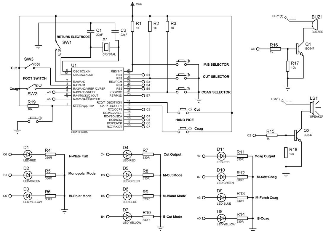
Fig 3.6 - Control and safety circuit with audio tone generator and modes selector.
