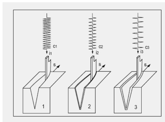
Fig 2.12 - HF current waveform
