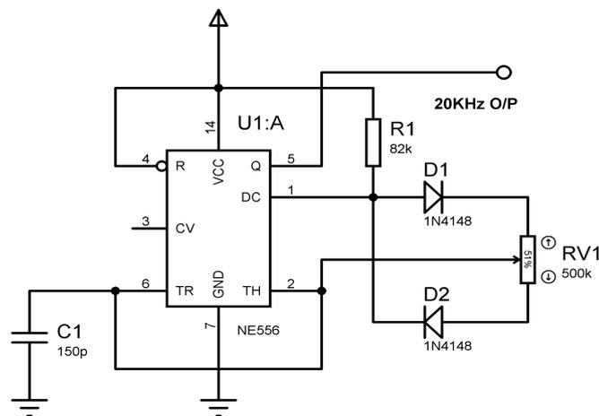
Fig 3.3 - 20KHz oscillator circuit
