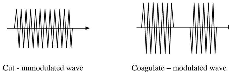
Fig 2.6 - Modulated and un-modulated wave
