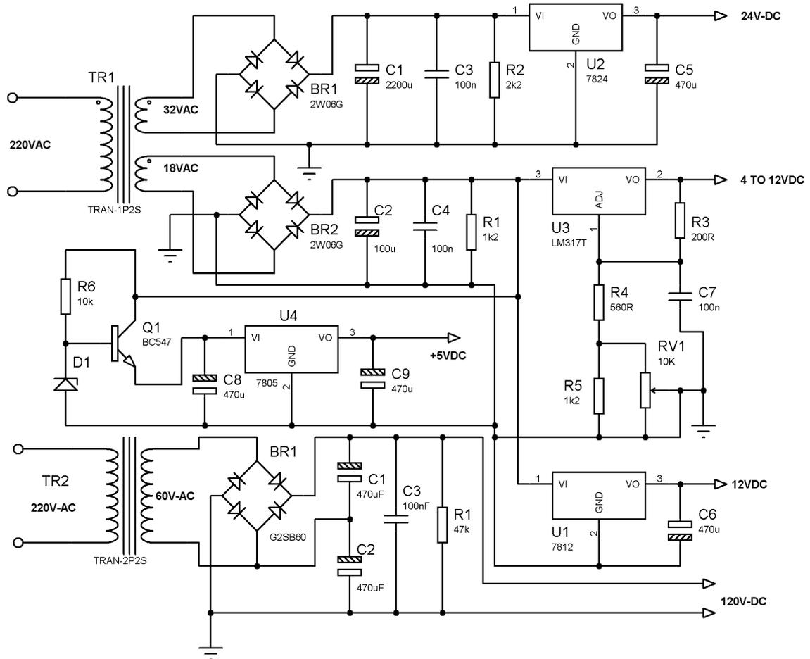
Fig 3.13 - DC power supply circuit.
