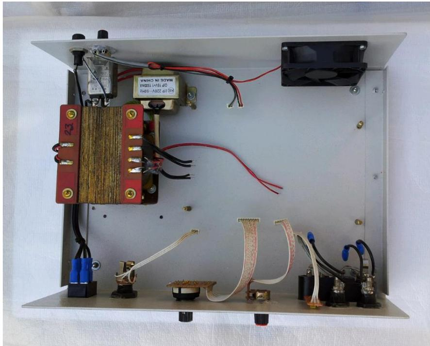
Fig 3.24 - Electro Surgical Diathermy Box with box fittings
