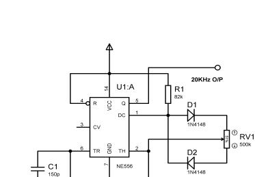
Fig 3.3 - 20KHz oscillator circuit
