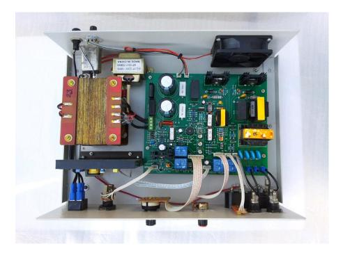
Fig 3.25 - Complete Electro Surgical Diathermy Machine
