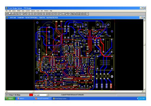
Fig 3.16 - Main PCB of Electro Surgical Diathermy
