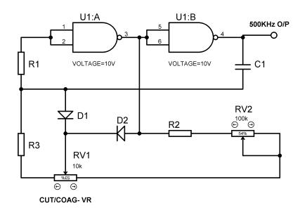
Fig 3.4 - 500KHz oscillation circuit
