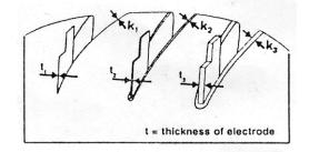
Fig 2.9- shape of the cut electrode used
