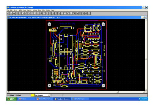
Fig 3.17 - PCB design Of 3 pin hand piece control circuit
