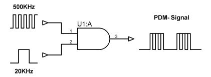
Fig 3.5 - Pulse duration modulation circuit
