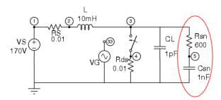
Fig 3.10 - Inductive Load Circuit
