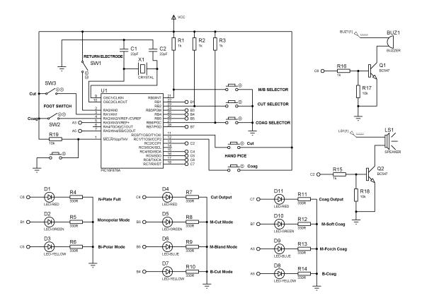
Fig 3.6 - Control and safety circuit with audio tone generator and modes selector.
