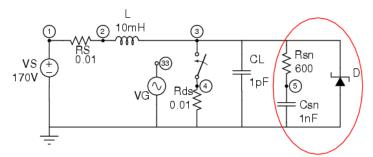
Fig 3.12 - Inductive Load Circuit with Snubber and Zener Diode
