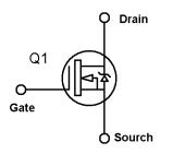
Fig 3.8 - N Channel MOSFET driver.
