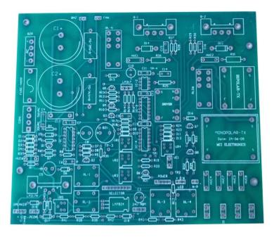
Fig 3.18 - Top Side of Electro Surgical Diathermy PCB
