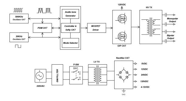
Fig 3.1 - Functional Block diagram of ESD machine
