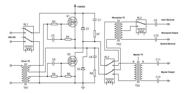
Fig 3.7 - HF Alternating Current Output Circuit
