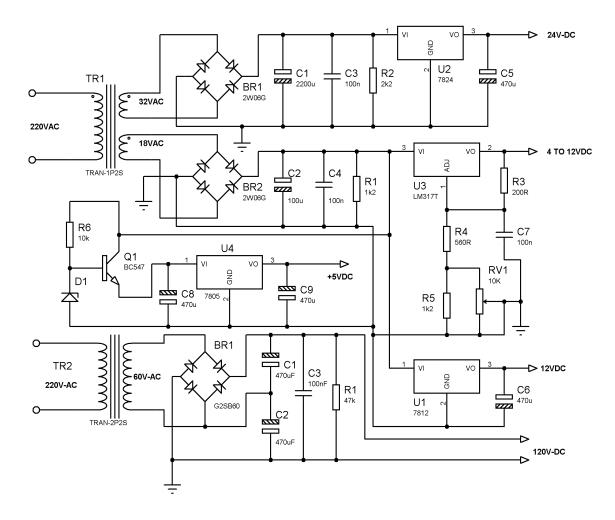
Fig 3.13 - DC power supply circuit.
