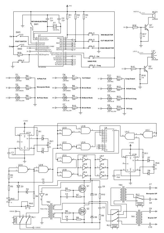
Fig 3.2 - Circuit diagram of ESD machine
