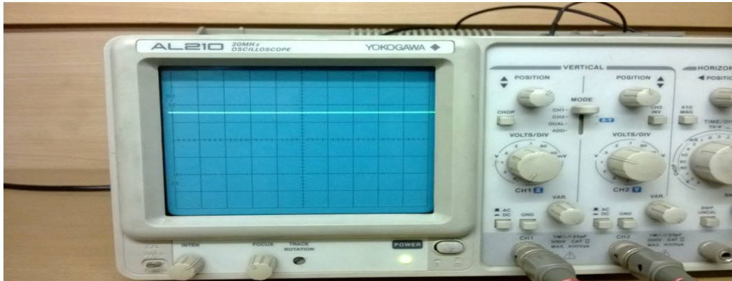
Output voltage L7806CV
