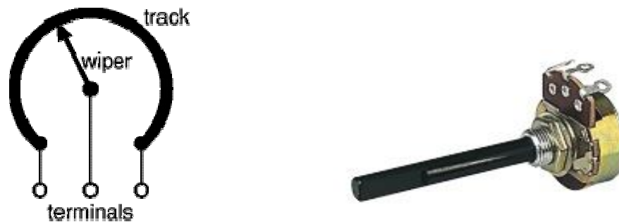
Fig 3.11 Internal and external construction of variable resistors [7]
