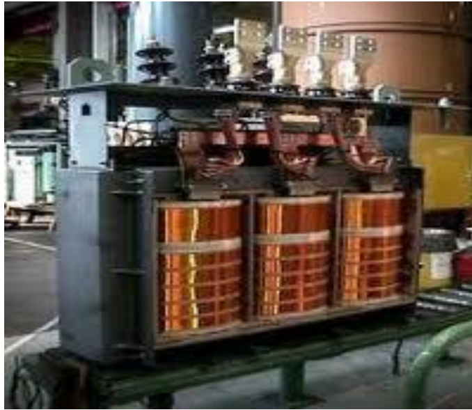
Fig: 6.1 Transformer core
