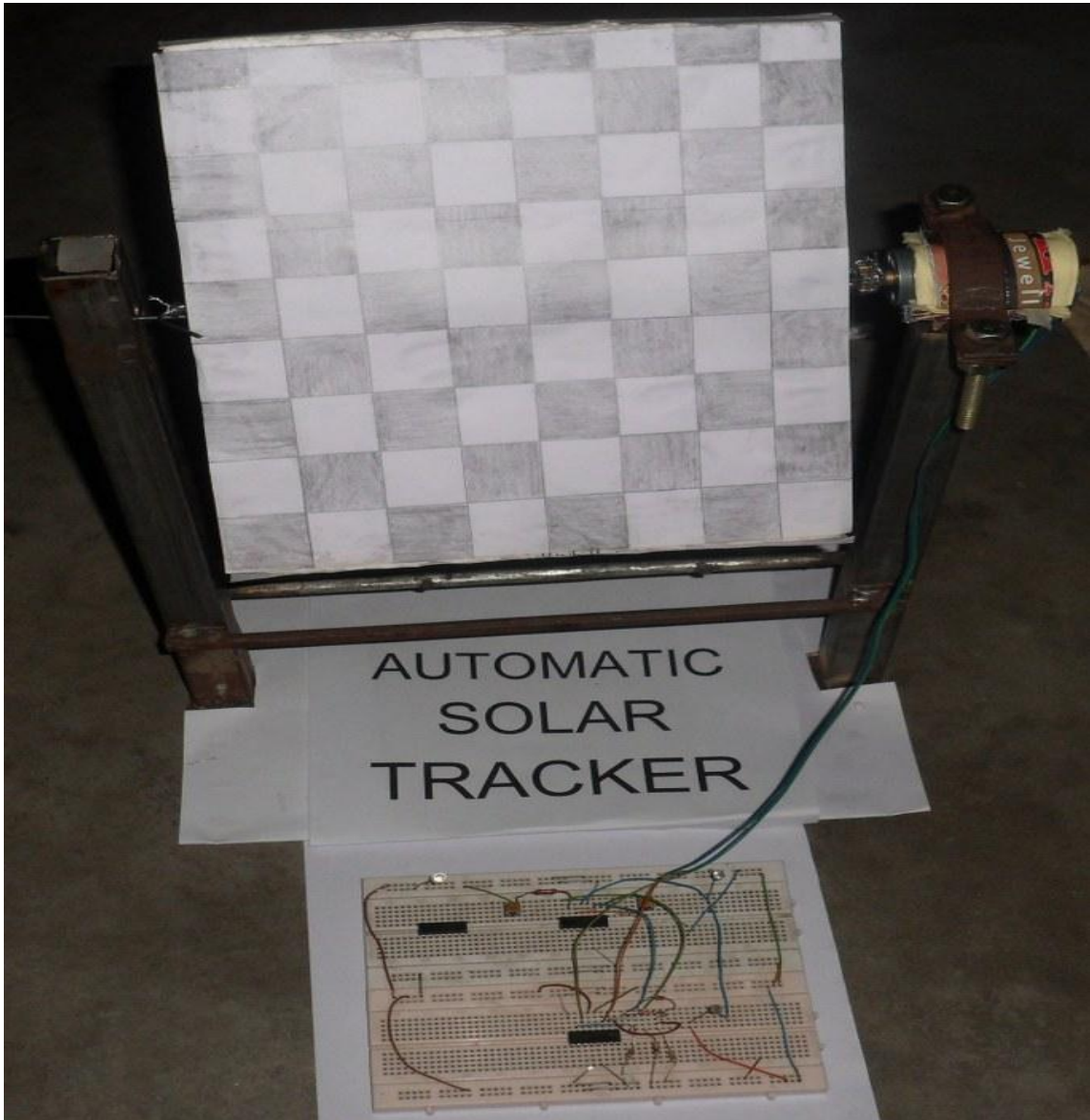
Figure 09: Proposed assembly for the Automatic Solar Tracker
