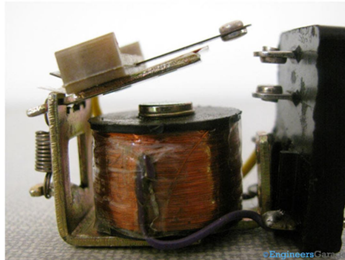
Fig 2.6: Internal Structure of Relay
