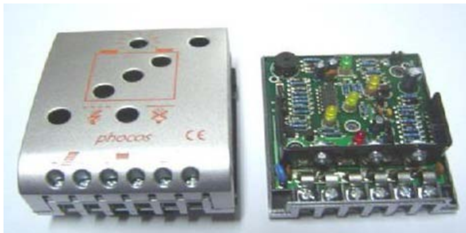
Figure: Charge controller
