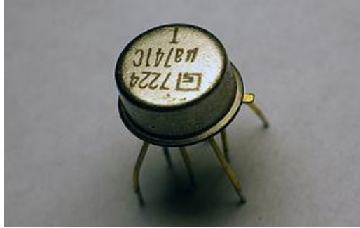
Fig-1.13: A Signetics \mu A741 operational amplifier, one of the most successful op-amps.
