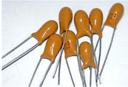
Fig-2.3: Solid-body, resin-dipped 10 \mu F 35 V tantalum capacitors.
