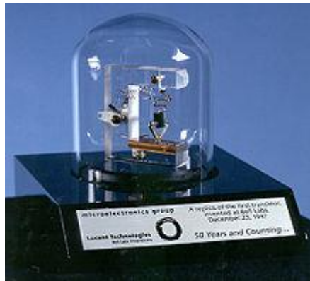
Fig 2.1: A replica of the first working transistor.
