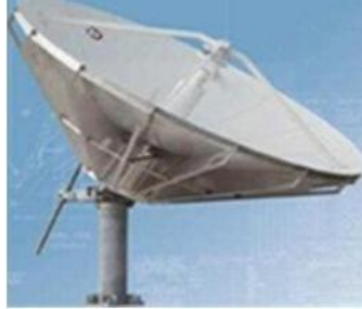
Figure 6.9 Parabolic Dish Antenna
