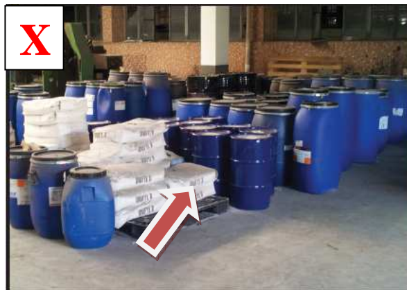
Figure 58: Liquid and solid chemicals improperly stored
