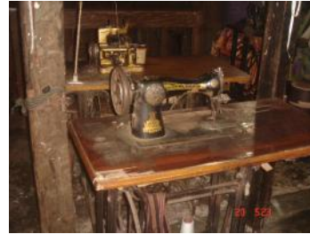
Figure - 47: Manual overlock machine. Figure - 48: Plain sewing (Lock stitch) machine.
