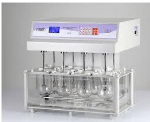
Fig 6-Dissolution apparatus.
