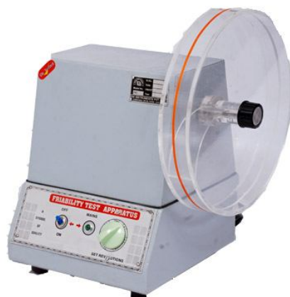
Figure 2.2: Friability test apparatus used for friability test
