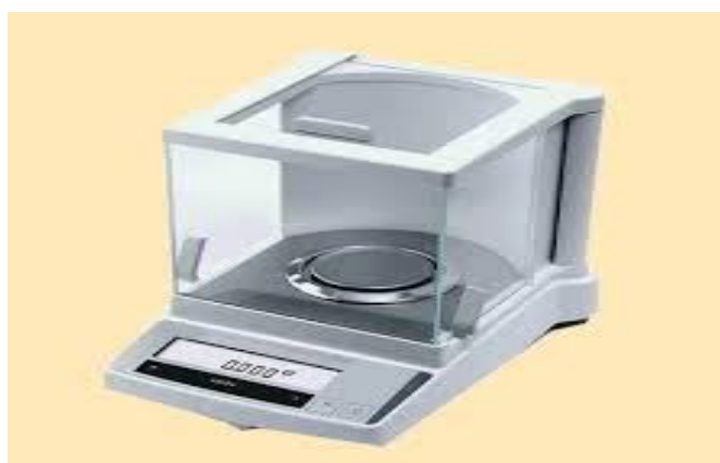
Figure 2.1: Analytical balance used for weight variation test
