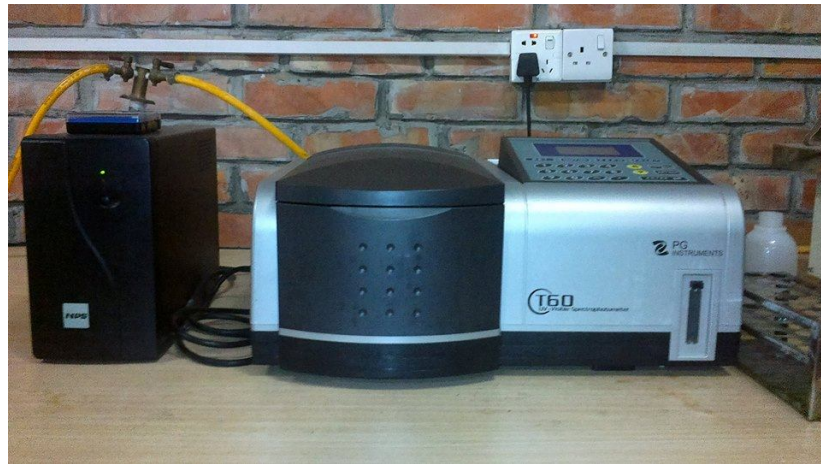
Figure 2.6: UV spectroscopy used for measuring the absorbance
