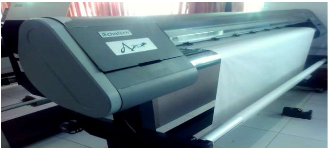
Fig: Marker making machine ( Wintex Plotter M/C)
