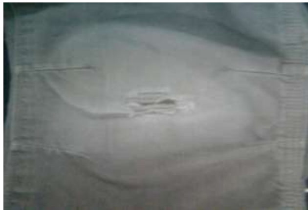
Fault of sand blasting:
