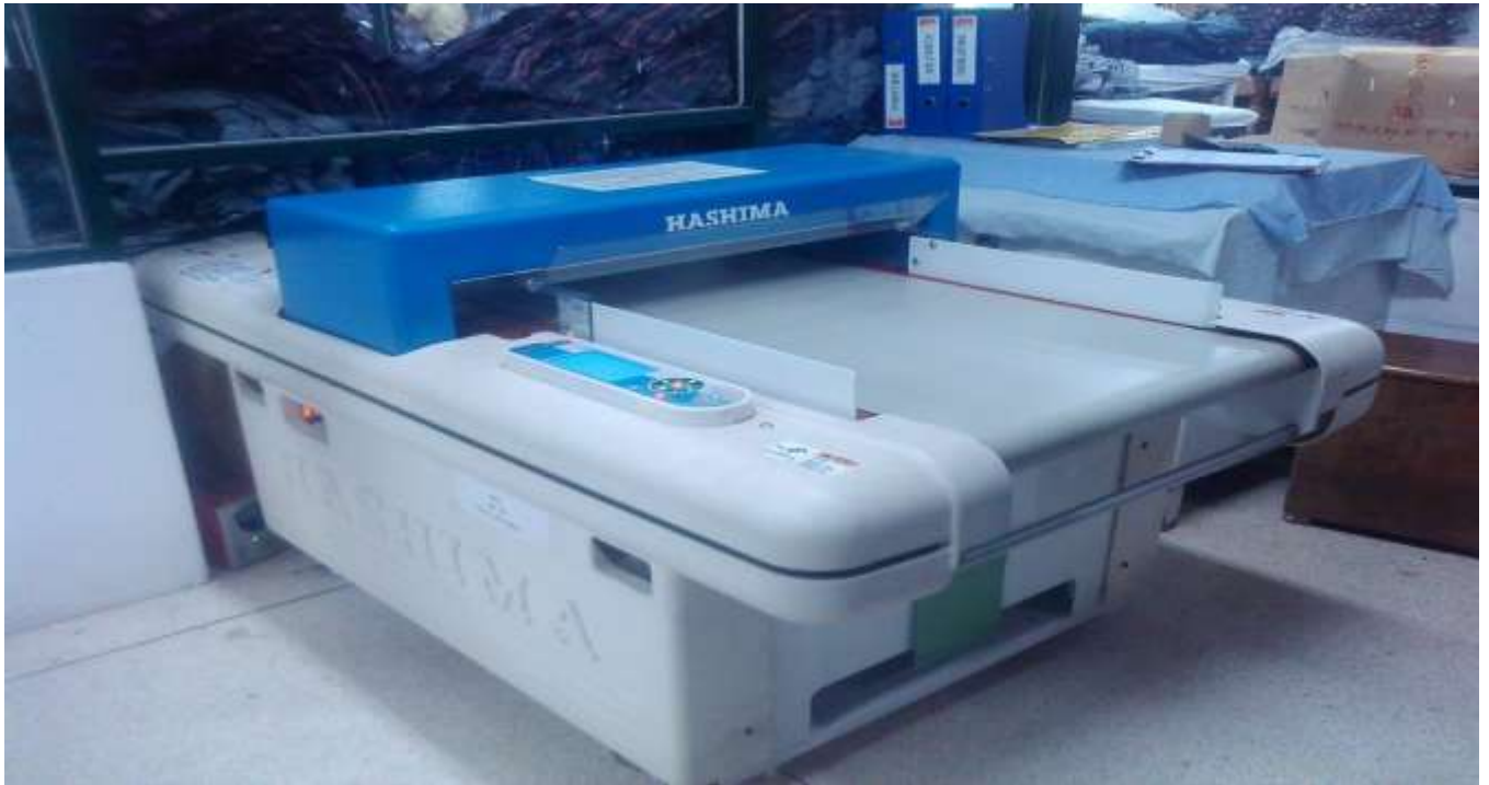
Fig: Metal Detector M/C(Brand name: HASHIMA)
