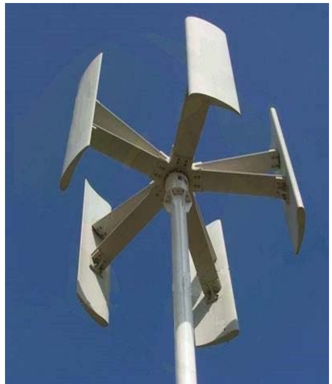
The 5 bladed H-TYPE or Gyromill wind turbine is variation of the Darrieus-type wind turbine.
