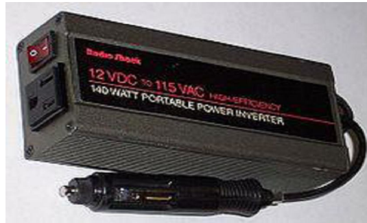
Figure2.17: Inverter designed to provide 115 VAC from the 12 VDC source provided in an automobile. The unit shown provides up to 1.2 Amps of alternating current, or just enough to power two sixty watt light bulbs
