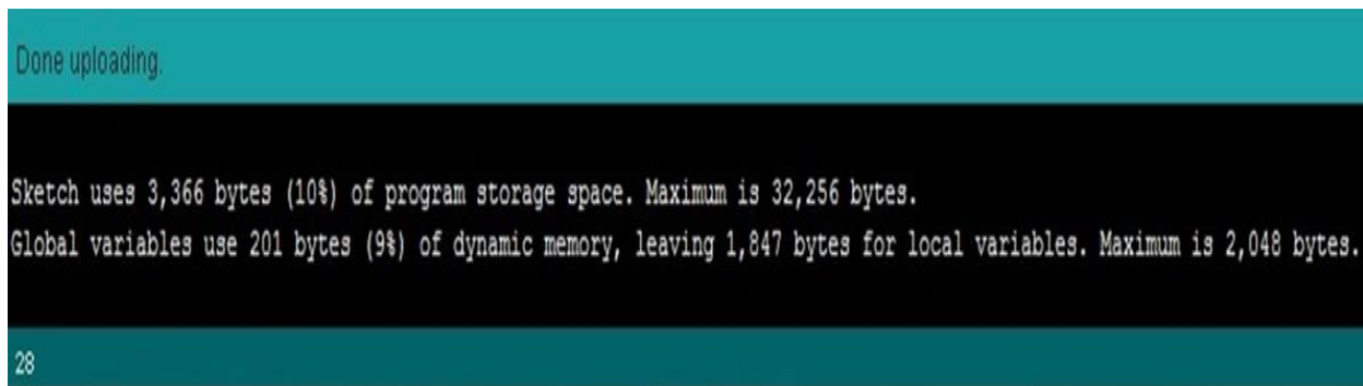
Fig 3.12: Message for upload complete
