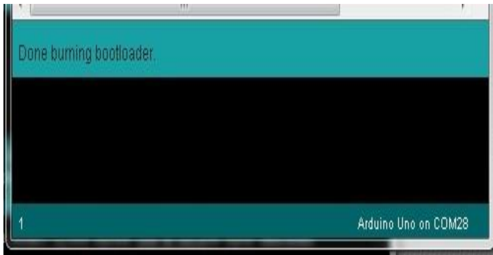
Fig 3.10: Confirmation message for burn Boot loader
