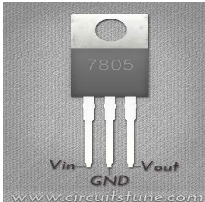
Fig: 2.2: Pin out of 7805
