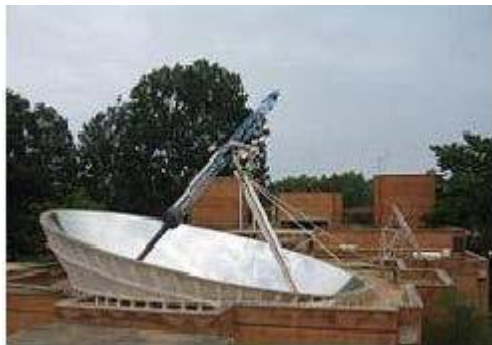
Fig3 : Solar cooking dish
