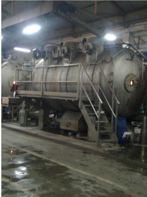
Figure: Fabric dyeing machine
