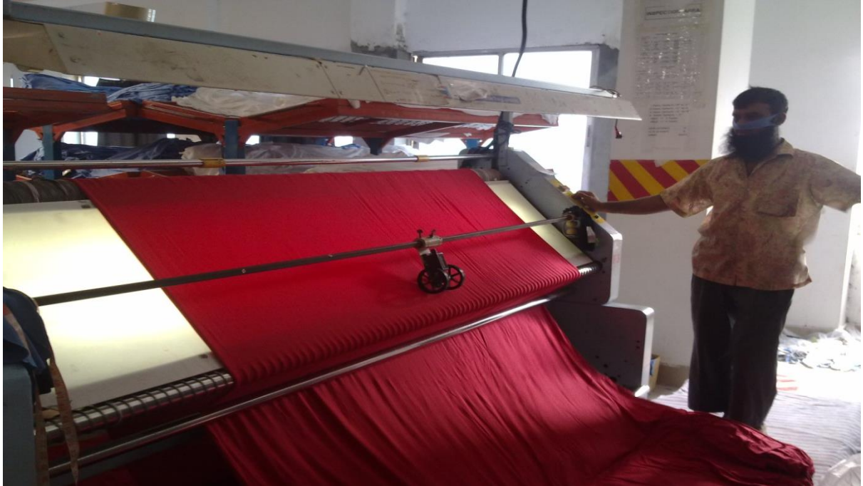
Fig: 4 – point system inspection
