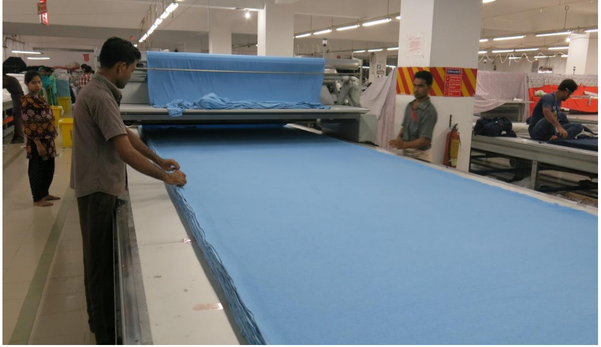
Fig: Automatic Spreading
