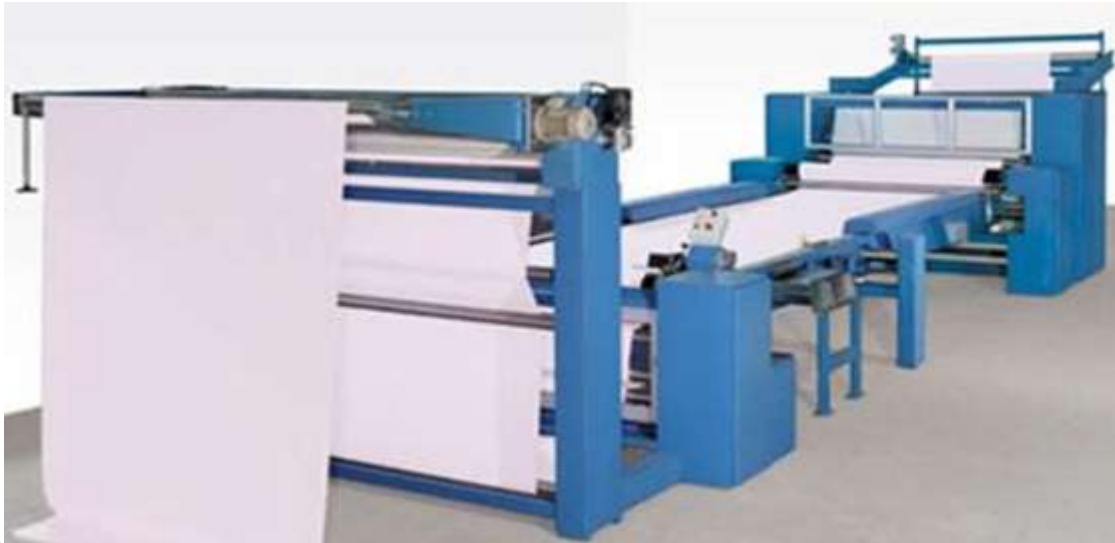
Fig:: Compactor machine.
