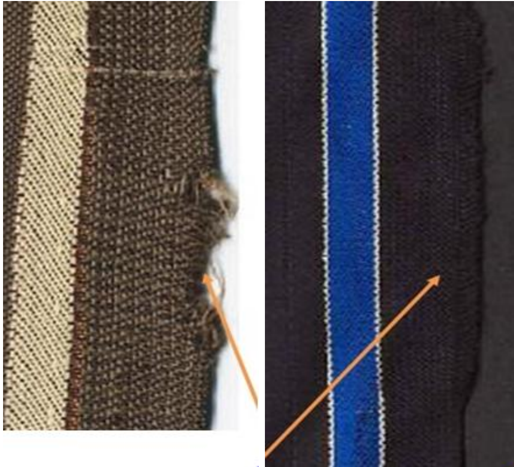
Figure 27: Cut or torn selvedge.
