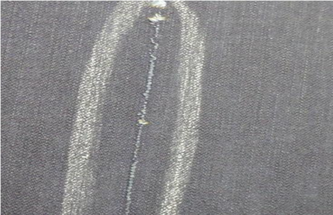
Figure 10: loose warp in fabric.
