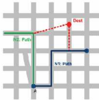
Fig 3.31: Calculation of the Nearest Point from packet's Destination for N1 and N2 [4]
