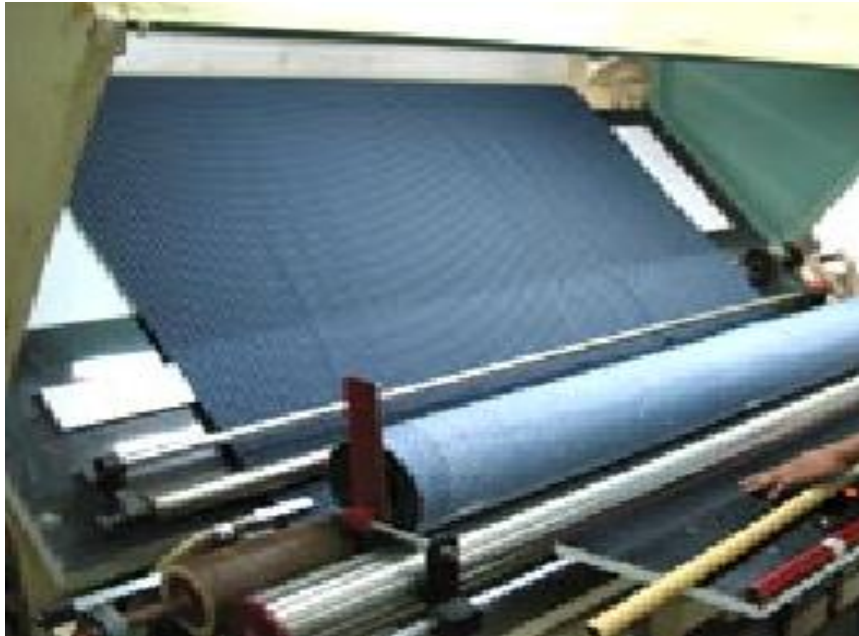
Figure 04: Fabric Inspection machine at Babylon Group.
