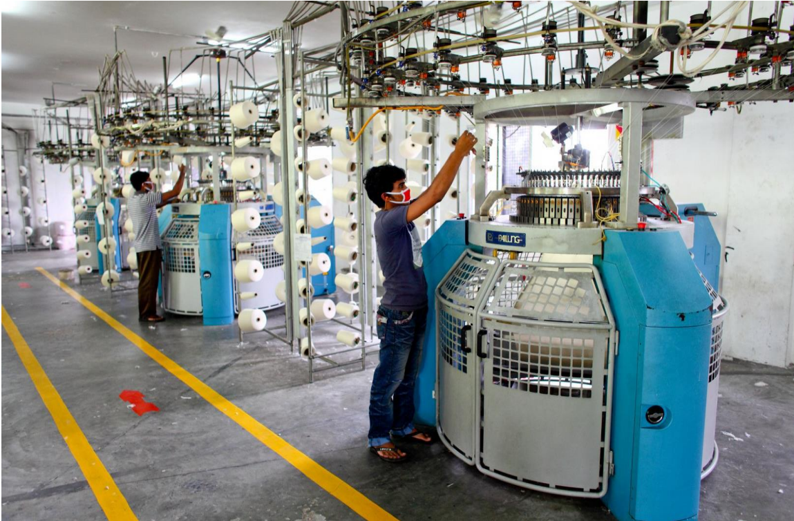
Figure 3: Double jersey knitting machine (interlock)
