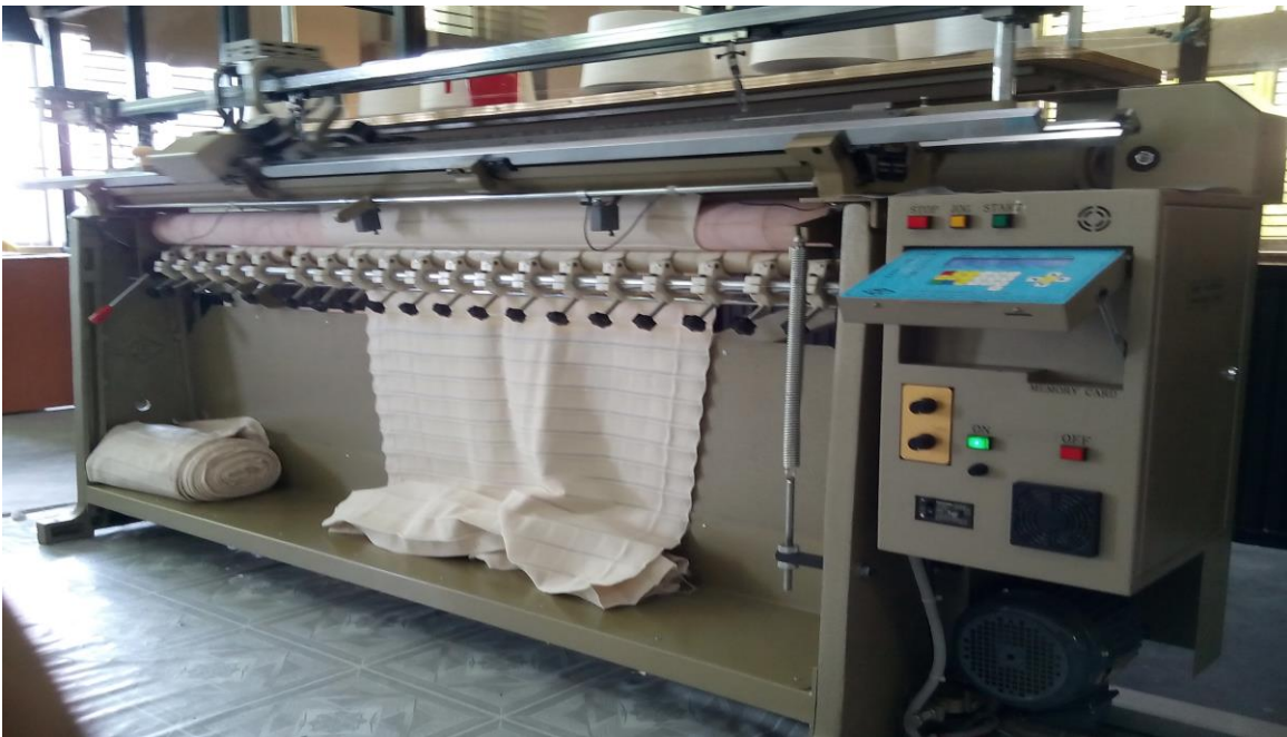
Figure 3: Double jersey knitting machine (interlock)
