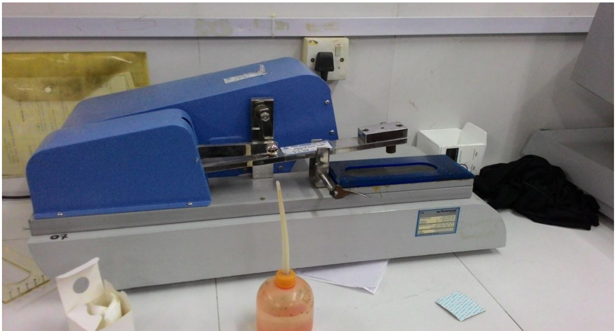
Fig: Crock meter For Rubbing Test
