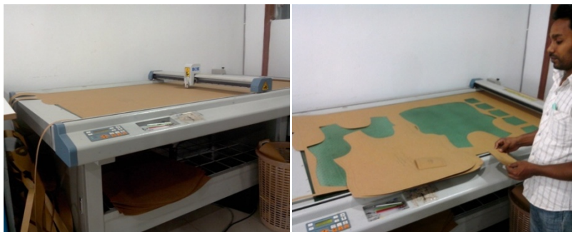
Figure 3.3.6 Patterns are cut by automatic pattern cutter & Supervisor is collecting the cut pattern
