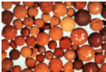
Figure: Shows a resin fouled with iron.
