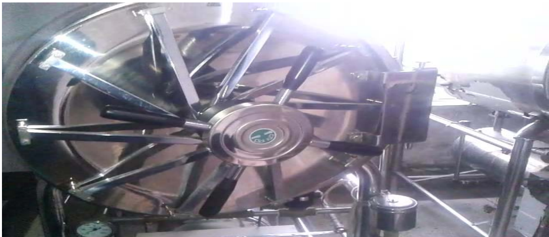
Figure 19: front view of autoclave machine(Jahurul islam medical college and hospital, bajitpur, kishoregonj.)
