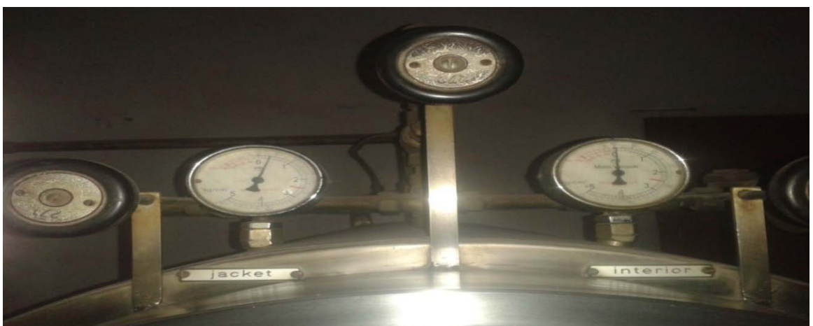
Figure 25: temperature meter of autoclave machine. (Holy Family Red Crescent Medical College, Dhaka.)
