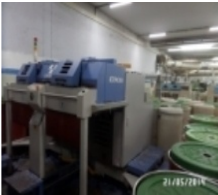
Model: Toyoda DX8 (Finisher draw frame) Origin: Japan Type: Auto Leveler & Double Delivery
