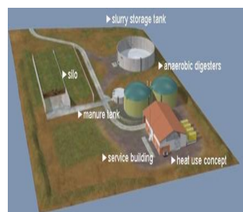
Fig:27 Biogas energy plant
