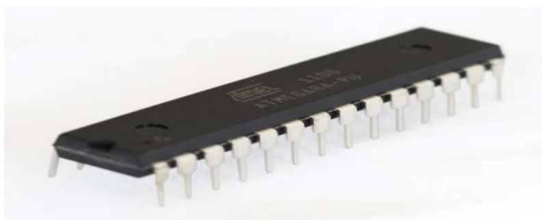
Fig: 3.1 ATMEGA8 28 pin Microcontroller
