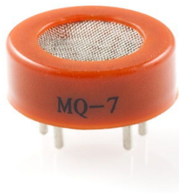
Fig: 5.1 Carbon- Monoxide Sensor (MQ-7)
