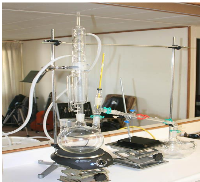
Figure (2.2): Soxhlet apparatus
